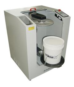
Programmable time and speed functions enhance mixing capabilities to satisfy the requirements of the selected base achieving a complete dispersion of colorant in the final product. There are three pre-set cycles and two additional customizable ones, allowing for mixing speed ranges of 95 to 180 rpm.
